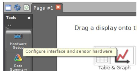
An image of the interface will pop up in the hardware setup window. On the interface click on the digital channel that the rotary motion sensor is plugged into. A window will pop up with a selection of different sensors. Scroll down and select the rotary motion sensor.
