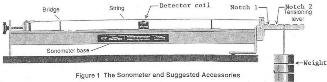
Figure 1 The Sonometer and Suggested Accessories
