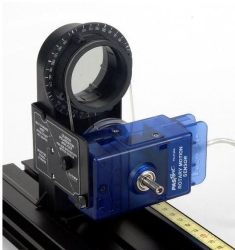
Figure 6: Rotary Motion Sensor Connected to Polarizer with Belt
