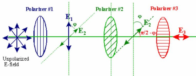
Figure 3: Electric Field Transmitted through Three Polarizers
