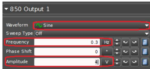
Click Record and observe the action of the meter. In turn, select each of the 8 AC waveforms and sketch the voltage outputs as a function of time of each waveform. Click STOP. Explain what is occurring to the voltage as a function of time of each waveform.
