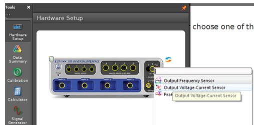
Drag a digits display to the screen and in **Select measurements** you can select either the internal voltage or current output of the interface.
