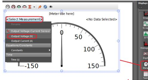
The meter display window opens with a center zero meter. Program the interface output for 4 V AC amplitude, sine wave output, and a frequency of 0.3 Hz.
