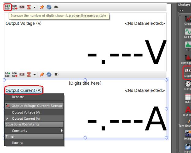
Set the analog voltmeter to 10 V DC. Next click on the signal generator icon and program the interface output for 10 V DC and click Record. How do the readings of the output voltage digits display, the voltmeter, and the programmed voltage, compare? Explain. Click Stop.
