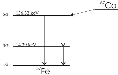
Figure 2: The energy-level diagram of the  $^{57}\text{Fe}$  nucleus.
