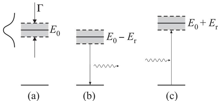
Figure 1: (a) Nuclear energy level has a half width  $\Gamma$ . (b) Shift in energy of emitted photon due to recoil of nucleus. (c) Shift in energy of absorptive transition because of the need of the absorbing nucleus to recoil. If the shifted levels (b) and (c) overlap, resonance fluorescence can occur.
