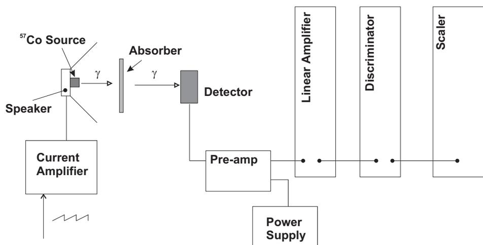
Figure 3: Schematic diagram of the apparatus.
