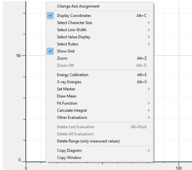
One item, **Energy Calibration**, will be of particular importance. To the left of the graph is a table which, when one or more energy spectra have been recorded, and this gives the counts for each channel of each run.
