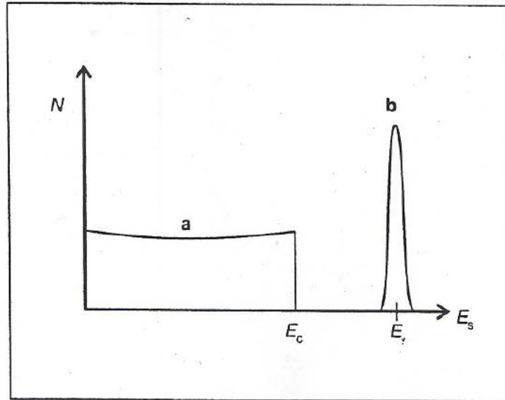
Figure 2: Histogram of a simplified pulse height distribution of a scintillation counter when monoenergetic  $\gamma$  radiation is absorbed. (a) Compton distribution (b) total absorption peak.
