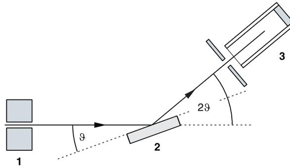
Figure 3: Diagram showing the basic components of the x-ray experiment. 1. Collimator, 2. Sample and 3. Detector slit and x-ray counter. In this experiment the incident and scattered angle are not necessarily equal.
