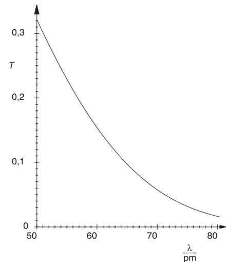
Figure 2: Transmission of a copper foil ( $d = 0.07$  mm) in the wavelength range from 50 to 80 pm. Figure from Leybold physics leaflet P6.3.7.1.
