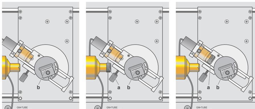
Figure 4: Experimental setup for Compton scattering. **Left:** without Copper filter, **Center:** with Cu filter (a) in front of Al scattering body (b), **Right:** with Cu filter behind the Al scattering body (b). Figure from Leybold leaflet P6.3.3.7.
