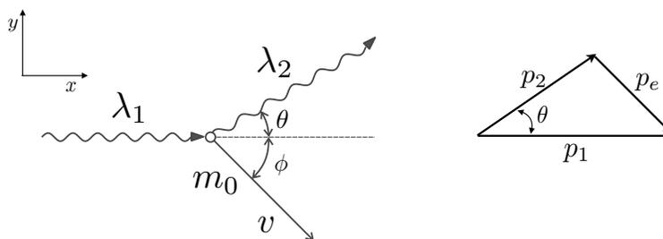
Figure 1: Compton effect. Left: An x-ray photon incident on a particle (an electron in this experiment) is scattered through an angle  $\theta$ . The initial wavelength of the x-ray is  $\lambda_1$  and the scattered x-rays wavelength is  $\lambda_2$  ( $\lambda_2 \geq \lambda_1$ ). The particle, initially at rest, acquires a velocity  $v$  in the scattering process. Right: Conservation of momentum in scattering process.
