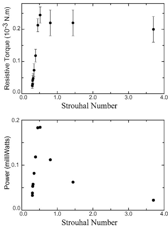
FIG. 9. In the presence of an external damping, and at fixed flapping amplitude ( $a=1.57$  cm) and frequency ( $f=2.5$  Hz), we study the response of the system to different external loads. We here show the torque ( $T_{\text{res}}$ , top figure), and the power produced ( $T_{\text{res}}\Omega$ , bottom figure), vs the Strouhal number.
