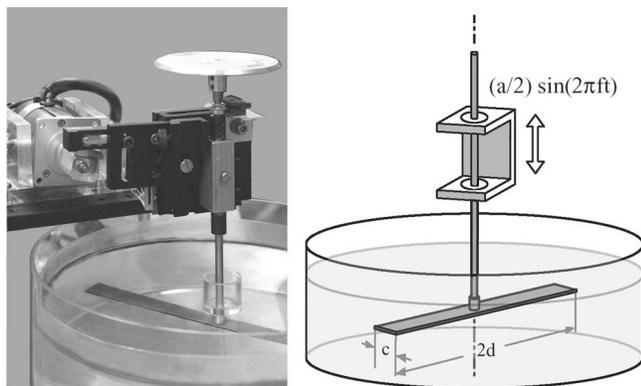
FIG. 1. The experimental setup. A rigid, rectangular wing is flapped up and down sinusoidally. It is allowed to rotate freely in the horizontal plane. The total length of the wing ( $2d$ ) is 25.7 cm, its width (chord,  $c$ ) 1.9 cm, and its thickness 0.16 cm. Both flapping amplitude and frequency can be adjusted to study the response of flapping motion of the wing and its surrounding fluid (water). A photograph taken from the setup is shown on the left and the schematic is shown on the right.
