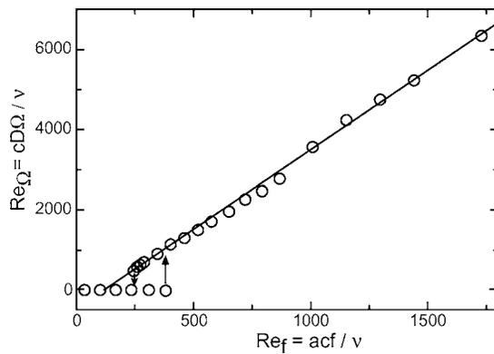
FIG. 2. Relationship between flapping frequency and rotational speed. When the flapping amplitude is fixed at 15.7 mm, the resulting forward-flight speed  $D\Omega$  is a linear function of the flapping frequency. Hysteresis is seen near the onset, likely due to the finite friction at the shaft.
