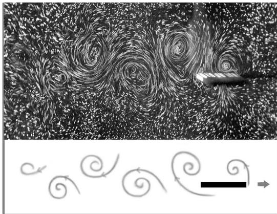
FIG. 3. Flow visualization around the flapping wing. A vertical light sheet is introduced into the fluid tank at position near  $D$ . The wake of the flapping wing that is in forward motion exhibits an “inverted” von Kármán vortex street. The corresponding illustration of the flow directions is sketched at the bottom.
