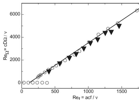
FIG. 5. The effect of flapping amplitude (shown as  $Re_f$ ) on rotational speed ( $Re_\Omega$ ): At a fixed flapping frequency,  $f=2.5$  Hz, the flapping amplitude is adjusted incrementally to change the driving Reynolds number  $Re_f$ . The resulting terminal speed of the forward-flight wing (solid triangles) follow closely the data obtained as one changes the frequency only (circles, same data shown in Fig. 2). The amplitude changes from 0.73 to 2.54 cm, which is 0.38 to 1.32 chord length.
