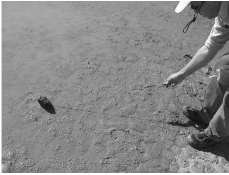
Fig. 6. Measuring the drag on a rock at Bonnie Claire Playa. Even though the mud felt extremely slippery underfoot, the weight of the rock causes it to sink through this lubricant and grip the rigid mud beneath, resulting in a measured coefficient of friction of 0.5 or more.
