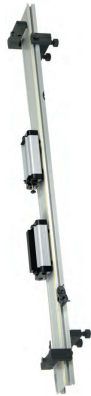
Figure 4.2 Low-friction track and carts used in the experiments described in this chapter.
