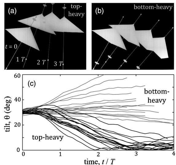
FIG. 4. Center of mass (c.m.) location and flight stability. Weights are added to the pyramid to make top- and bottom-heavy bodies. The pyramid height is 1.7 cm in both cases, and the c.m. is located at the apex and 1.5 cm below the base, respectively. The objects are released into the flow with tilt  $\theta = 30$  deg. (a),(b) A top-heavy pyramid recovers the upright orientation, while a bottom-heavy body tips over. (c) Body tilt dynamics for top- and bottom-heavy pyramids.
