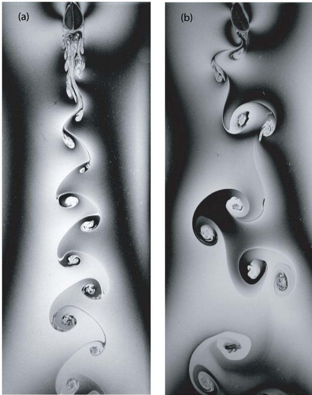
FIG. 1. Vortex wakes behind a flexible loop. (a) Wake structure after the stationary loop. (b) Wake structure after the oscillating loop.
