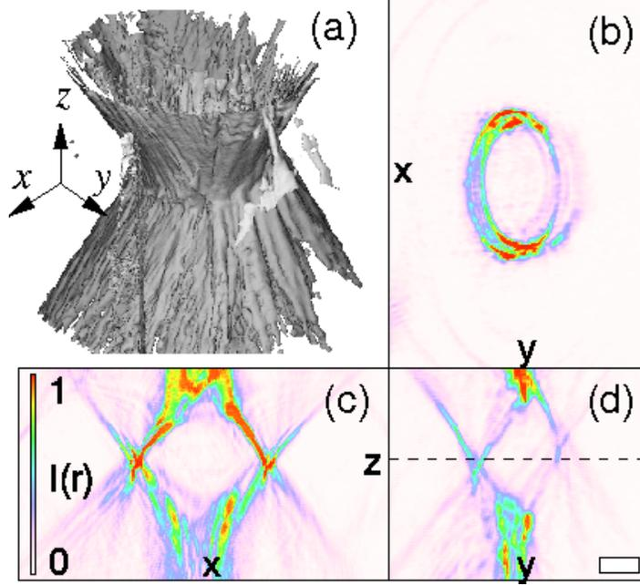
Fig. 2. (a) Volumetric reconstruction of a tilted ring trap. (b) Horizontal section near the midplane showing tilt around the  $\hat{y}$  axis. (c) Vertical section along the  $\hat{x}$  axis. (d) Vertical section along the  $\hat{y}$  axis.
