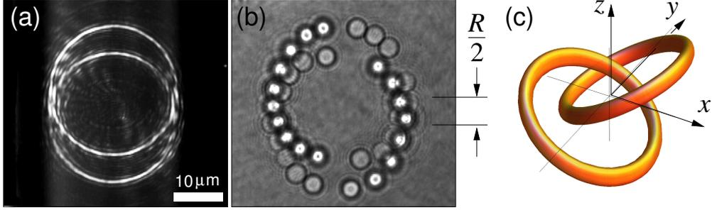
Fig. 4. (a) Intensity in the focal plane of the microscope of two tilted ring traps projected simultaneously with opposite inclination,  $\beta = \pm\pi/8$ . (b) Colloidal silica spheres trapped in three dimensions within the focused Hopf link. (c) Schematic representation of the three-dimensional intensity distribution responsible for the image in (a).
