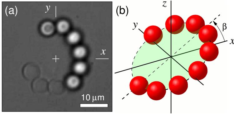
Fig. 3. (a) Bright-field microscope image of  $5.17 \mu\text{m}$  diameter colloidal silica spheres trapped on an inclined ring. (b) Schematic representation of the geometry in (a). The Media file shows particles circulating around the inclined ring under the influence of phase-gradient forces.
