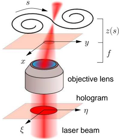
Fig. 1. Projecting three-dimensionally extended holographic traps. A laser beam is imprinted with a hologram in the input pupil of an objective lens. The hologram is projected through the objective’s focal plane, and comes to a focus along a three-dimensional curve parameterized by its arc length,  $s$ .
