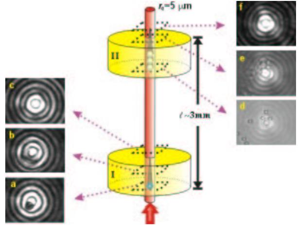
FIG. 8: The radial phase profile  $\varphi(\vec{\rho}) = \gamma\rho$  creates a diffractionless Bessel beam that focuses to a long axial trap. Here, the same beam is shown trapping multiple colloidal particles in two separate sample chambers separated by 3 mm. Distortions due to a particle trapped in plane (a) heal themselves in planes (b) and (c). The process is repeated for the same beam in planes (d), (e) and (f). From Ref. [86].
