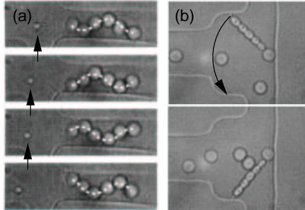
FIG. 5: Optical pump (a) and valve (b) constructed of colloidal particles in microfluidic channels activated with optical tweezers. The flow of water created by the colloidal peristaltic pump is visualized by the tracer particle indicated with an arrow. The colloidal valve flap is flipped with an optical tweezer and directs particles either downward (top) or upward (bottom). Adapted from Refs. [57] and [58].
